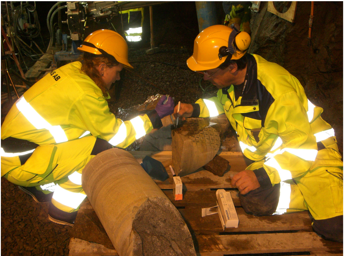
Figure 3-1. Sampling of a fracture surface for microbial presence by using DNA/RNA analysis methods within the Microbe Project.
