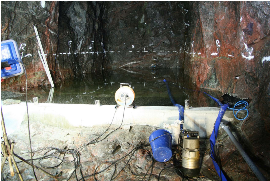
Figure 4-1. Inflow measurement in a weir in the Tass-tunnel for the project Sealing of Tunnel at Great Depth.
